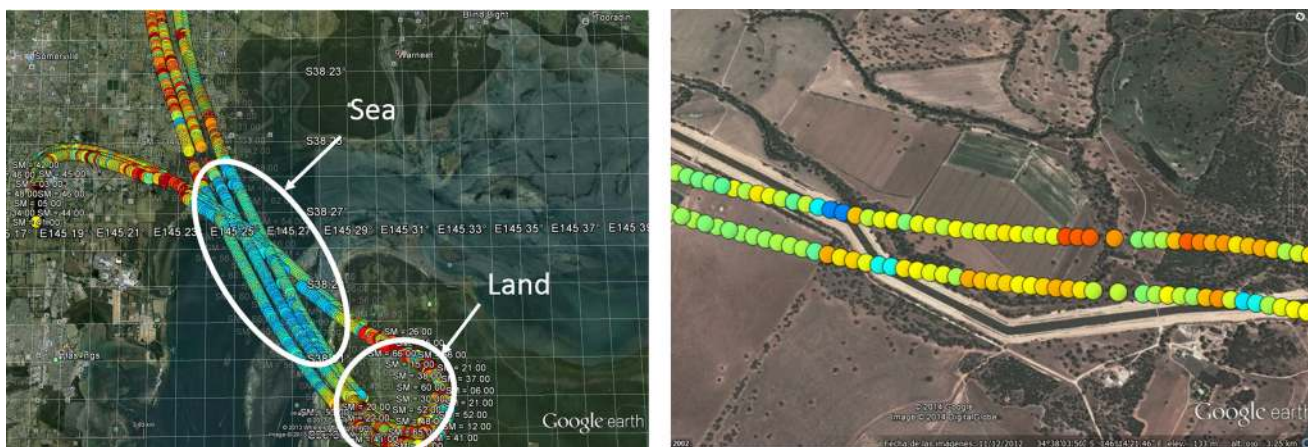
Fig. 28. Left: Sample ground-tracks of up to 4 simultaneous GNSS-R reflections after take-off Melbourne (Australia) collected with the LARGO instrument, and Right: sample ground-tracks showing the variability of the scattering coefficient over terrain and water bodies. The color scale represents the forward scattering coefficient (blue: high, red: low). The largest scattering is produced over water bodies, either the ocean (left image) or over water channels (right image). Over the ocean there is also variability due to different sea states (left). Over land (right plot), lower/higher scattering (red/blue) is associated with lower/higher soil moisture conditions (dry/moist soil). Surface roughness, vegetation, and topography effects also play a role in the magnitude of the scattering coefficient.
