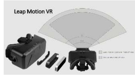
Figure 4: Oculus Rift and Leap Motion configuration
