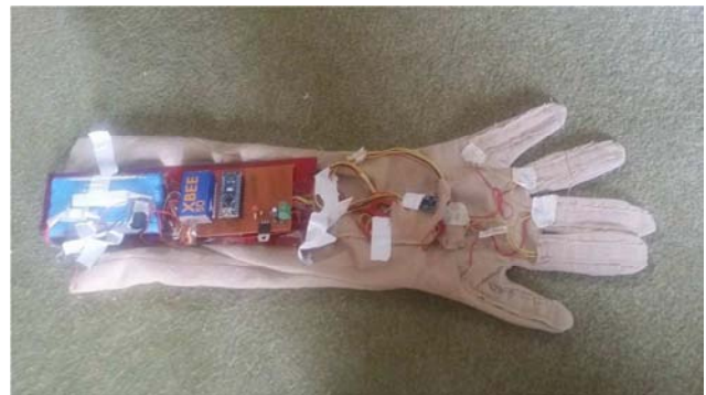
Figure 8. Complete Design of the human hand Glove.
