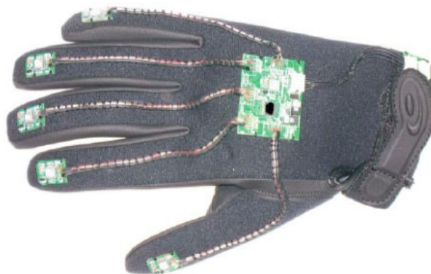
Figure 1. eGlove with motion sensors and CPU circuitry (Patents pending 12/323,986; 12/325,046)
