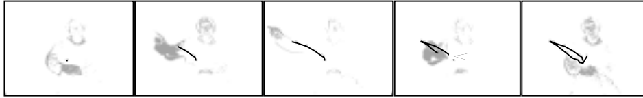
Figure 2: Selected temporal difference frames from the second sequence in Figure 1. The area of detected motion is shown as mid-grey here, whilst the path described by the estimated centroid is overlaid in black.
