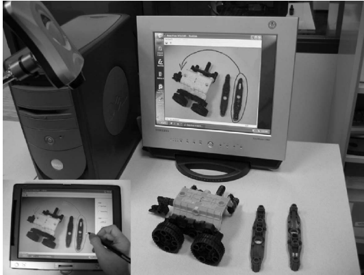
Figure 7. Close-up of the DOVE drawing tool on the Helper's tablet PC (left front insert) and on the Worker's monitor (right).
