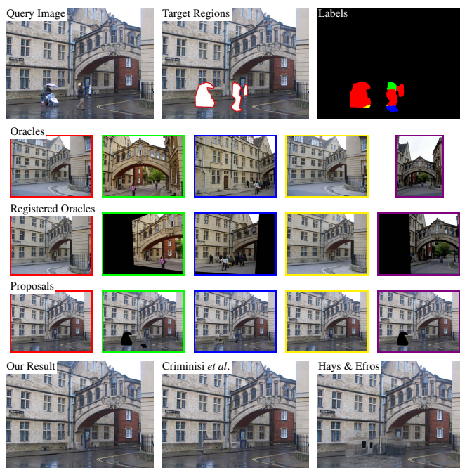
Figure 1: An overview of our system. Top row: The inputs to the system and the output labels showing the combination of proposals in the final result. Middle rows: The top 5 oracles used in the result and their proposals. Oracles are obtained automatically from the Internet using viewpoint invariant search. Last row: Our result, the result using the algorithm of Criminisi et al. [4] and the result using the method of Hays & Efros [7].
