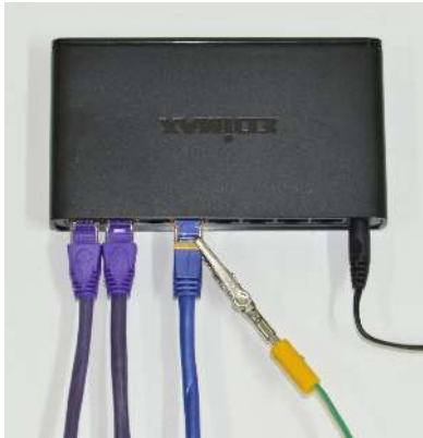
(a) Measuring shield potential at the far side of an Ethernet cable (probed at the Ethernet switch).
