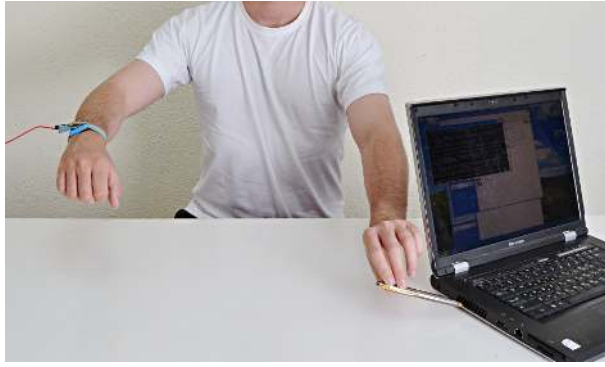
(a) Non-adaptive “human touch” attack through a metal pen touching the heatsink fins. The wristband is connected to the probe wire.
