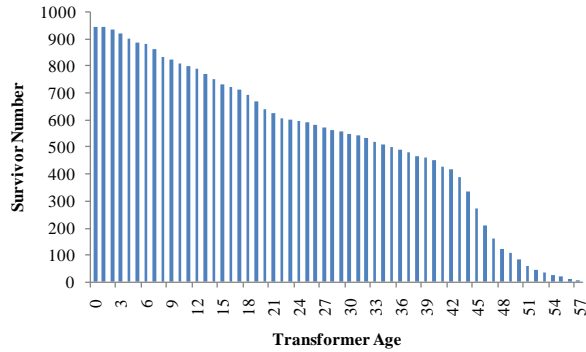
Figure 1. The UK transmission power transformer's survivor number from Age 0 to 57.
