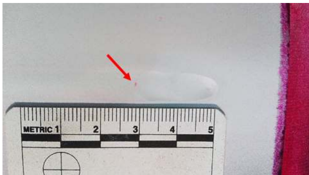
Fig. 17—Dye penetrant Indication on sample TVA 2.3 (X65 steel) where no cracks were observed during stereoscopic examination.
