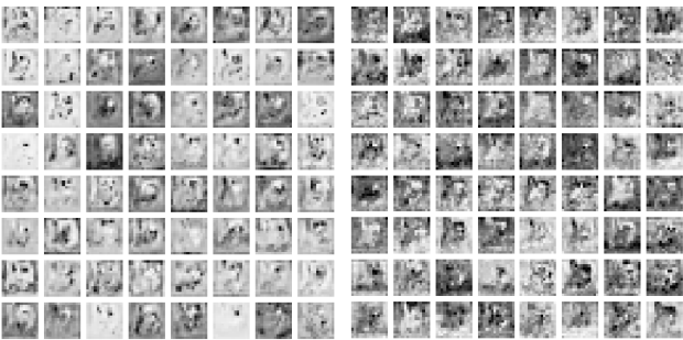
Fig. 13 The feature maps of the third stage of G-Ghost-ResNet34. Left: features from complicated path, right: features from cheap operation.
