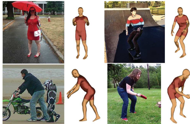
Figure 10. Monocular 3D human pose and shape reconstruction with GHUM by relying on non-linear pose and shape optimization under a semantic body part alignment loss.
