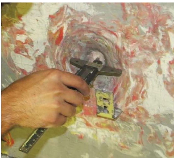
Figure 3. Measurement of the depth in the clay witness caused by the projectile impact. Source: authors.
