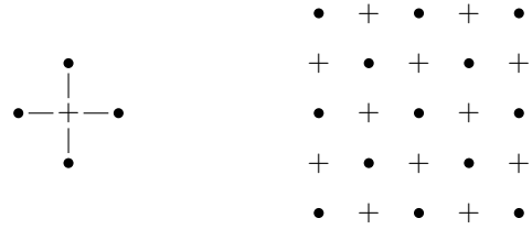
Figure 1. The four-element cross-neighborhood and the tessellation of the index set \mathcal{S} into two disjoint sublattices \mathcal{S}_e and \mathcal{S}_o .
