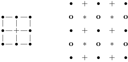
Figure 3. The eight-element neighborhood and the tessellation of the index set \mathcal{S} into four disjoint sublattices marked with four different symbols.
