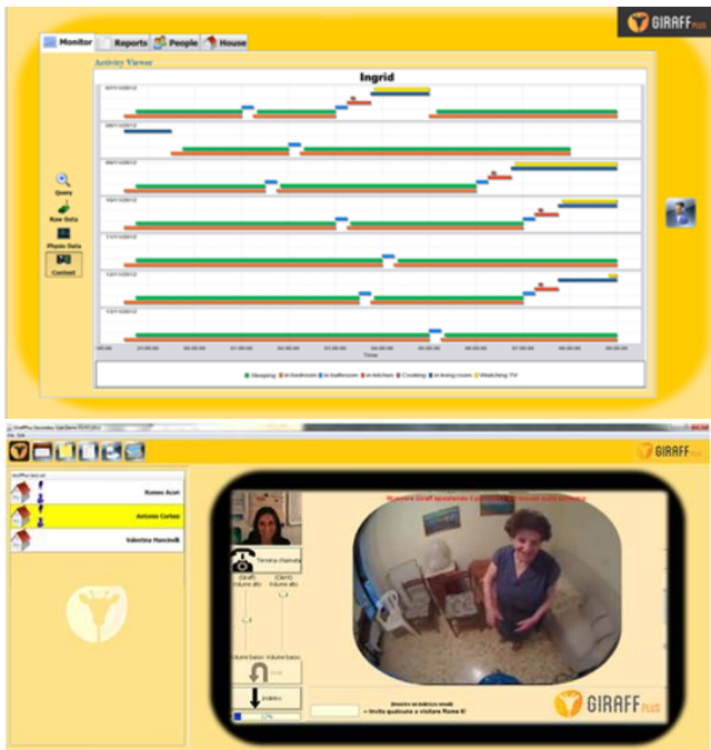
Fig. 5 Upper graph, visualization of night activities: green line - sleeping; orange line – in bedroom; light blue line – in bathroom; light red line – in kitchen; dark red line – cooking; dark blue line – In living room; yellow line – Watching TV. Lower display, interface for the remote driver of the Giraff robot
