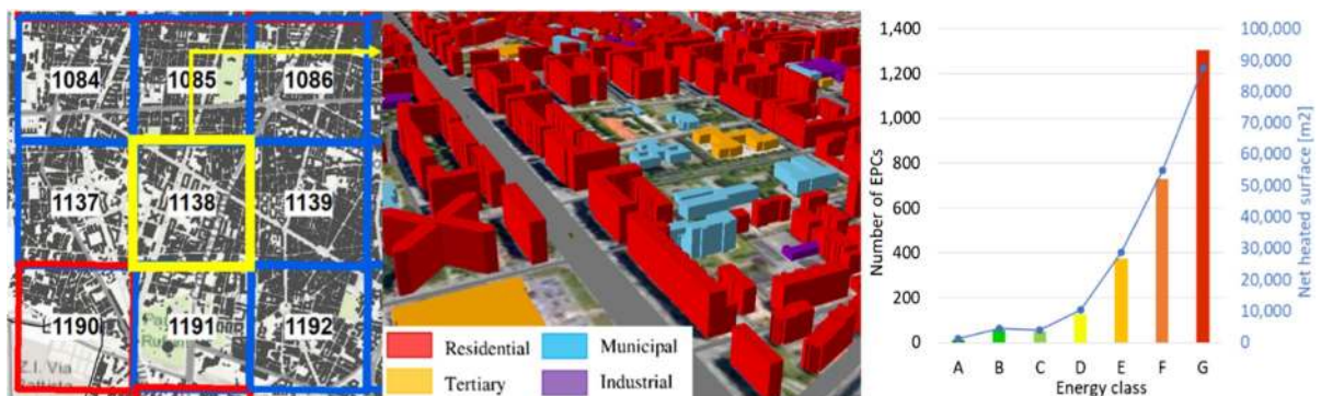
Fig. 2 Example of some aspects of the urban energy atlas: mesh identification; building classification according to the type of user; EPC data of the residential sector
