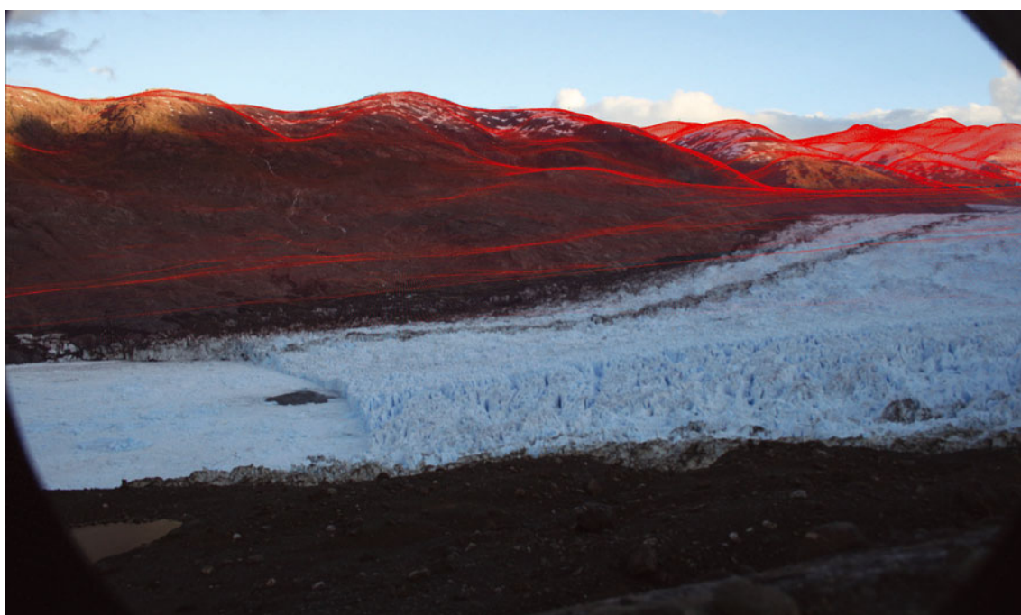
Fig. 3. Camera orientation determined by geo-referencing the photographs to a DEM (red lines) of the area. The black areas at the image corners are the shadows of the camera house.
