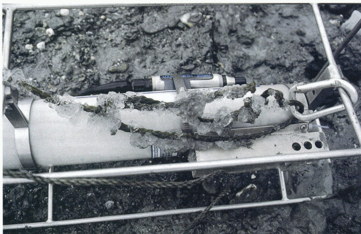
Fig. 6. Ice crystals, some in the form of rosettes, that grew on the rope and metal cage of an instrument (CTD unit) suspended in an active vent.
