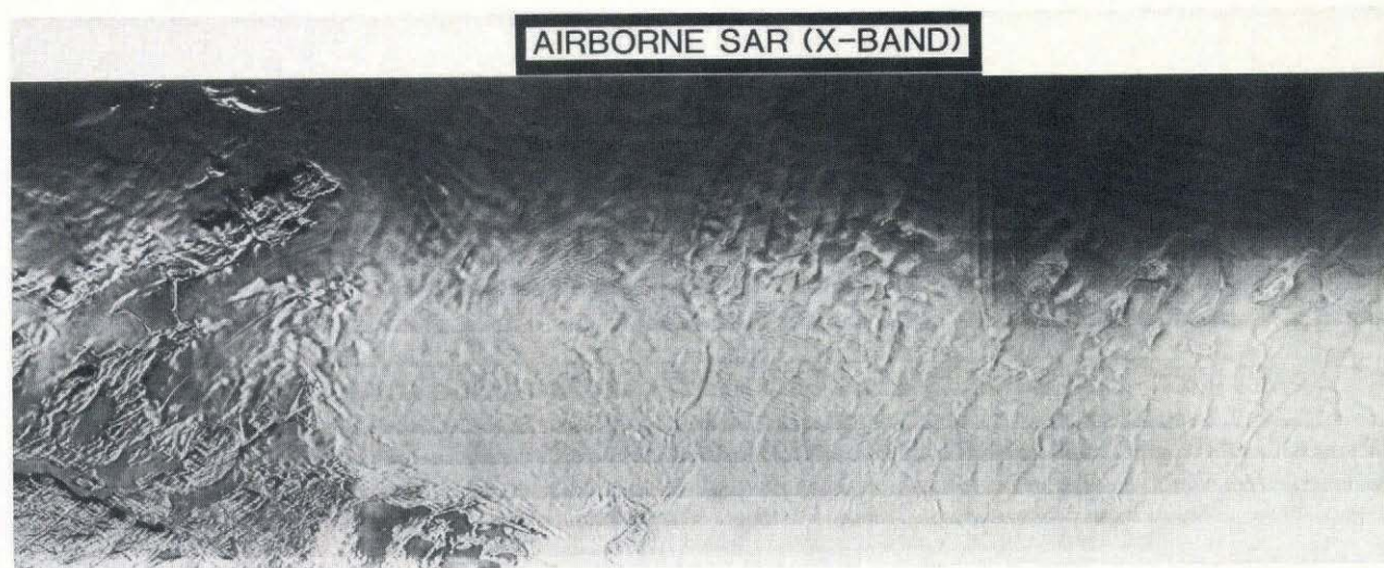
Fig.4. Western end of airborne SAR data in southern Greenland collected on 14 April 1986. Width of swath is approximately 45 km. Illumination is from the bottom. Antenna depression angle was 14^\circ over the left two-thirds of the image but was increased to 15^\circ over the remaining one-third of the image.
