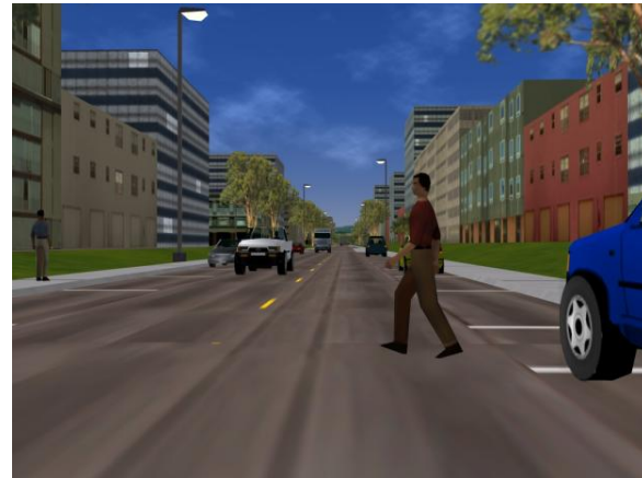
Figure 4. Simulated two-lane city road with lane markings and ambient traffic. The image also illustrates an unexpected event: a pedestrian walking into the roadway from behind a vehicle parked on the side of the road.
