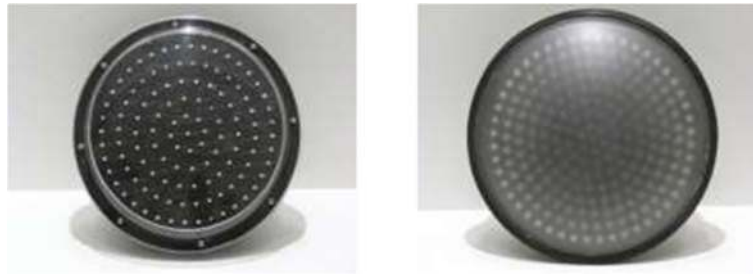
Figure 1 GLeds (left) and Mleds (right). Studied traffic lights with directly visible LEDs.
