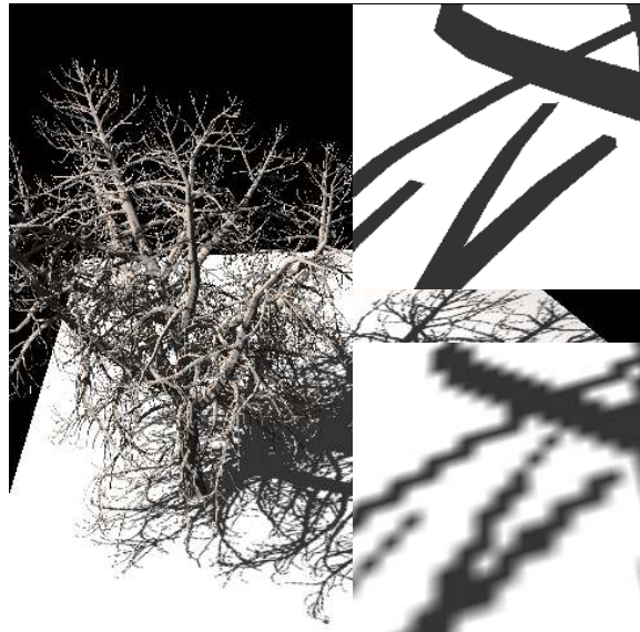
Fig. 7: This adaptive shadow map uses a GPU-based adaptive data structure built with the Glift template library. It has an effective shadow map resolution of 131,072^2 (using 37 MB of GPU memory, trilinearly filtered). The top-right inset shows the ASM and the bottom-right inset shows a 2048^2 standard shadow map.
