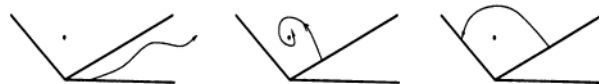
Fig. 3. Possible scenarios for a trajectory entering a cell: not convergent or unstable, stable, and switching trajectory.
