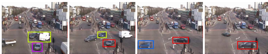
Figure 8: The local behaviours that contribute to the false detection of clip 9 as an anomaly using the standard pLSA.
