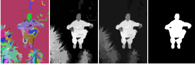
Figure 5. Image regions generated by Felzenszwalb and Huttenlocher’s segmentation method [11] (left), region contrast based segmentation with (left-middle) and without (right-middle) distance weighting. Incorporating the spatial context, we get a high quality saliency cut (right) comparable to human labeled ground truth.
