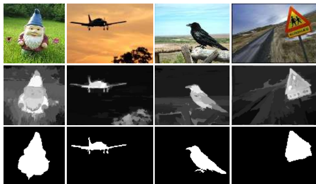
Figure 1. Given input images (top), a global contrast analysis is used to compute high resolution saliency maps (middle), which can be used to produce masks (bottom) around regions of interest.
