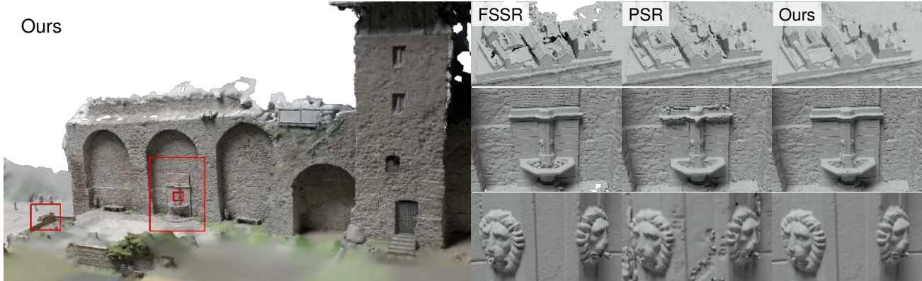
Figure 8. Reconstruction of the Citywall data set from [19] with 256 million points. Left: Colored reconstruction of the whole scene with our method. The annotations mark the three close-up views which are (top to bottom) the city model, the fountain and the lion heads. FSSR: FSSR generates a detailed reconstruction of the scene but has problems with holes in the city model and shows artifacts in the basin of the fountain. The artifacts are linked with the rest of the scene and cannot be removed easily. Of all methods, FSSR shows the best reconstruction near the mouths of the lion heads. PSR: The reconstruction with PSR contains many noise artifacts. Some artifacts could be removed with the provided clean-up tool in exchange for causing holes in the reconstruction as seen in the city model. The reconstruction of the lion heads is too smooth due to a maximum octree depth of 14. Memory did not permit a reconstruction using a deeper octree. Ours: Our method generates a surface without holes for the city model and preserves most of the concave structure between the houses. The basin of the fountain has some small artifacts. In contrast to FSSR, the view to the bottom of the basin is not blocked by reconstruction artifacts. The lion heads show all details but the surface of the taps of the lions is slightly underestimated. Results for SSD are not shown because the method did not finish after multiple days.
