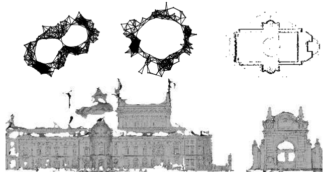
Figure 6. Opera dataset (160 images). Top: input epipolar graph (corrupted by façade symmetries), our cleaned graph, and calibration point cloud. Bottom: orthographic façade and close-up.
