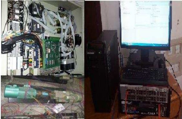
(a) Photograph of the experimental system with prototype PMSM Fig. 3. The schematic diagram of identification hardware and software platform.
