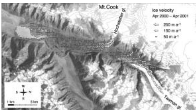
Figure 16 Ice flow vectors for Tasman glacier, New Zealand, ( 170^{\circ}10' \text{ E} , 43^{\circ}35' \text{ S} ) as derived from ASTER images of 29 April 2000 and 7 April 2001. The original 100 m spacing of the raw measurements is re-sampled to 200 m spacing. Ice speeds amount up to 250 \text{ m a}^{-1} . The marked- and surprising - decrease of ice flow for Tasman glacier at the confluence with Hochstetter glacier indicates a complex interaction between both glaciers. At the glacier terminus lake, a dashed line marks the lake extent of 7 April 2001 superimposed on the 29 April 2000m orthoimage. The observed lake growth towards the ice front amounts up to 130 m. From Kääb (2002).
