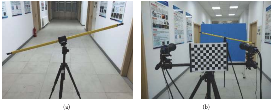
FIGURE 5: Target measurement experiment. (a) 1D long target with two feature points. (b) First measurement position of the cameras.
