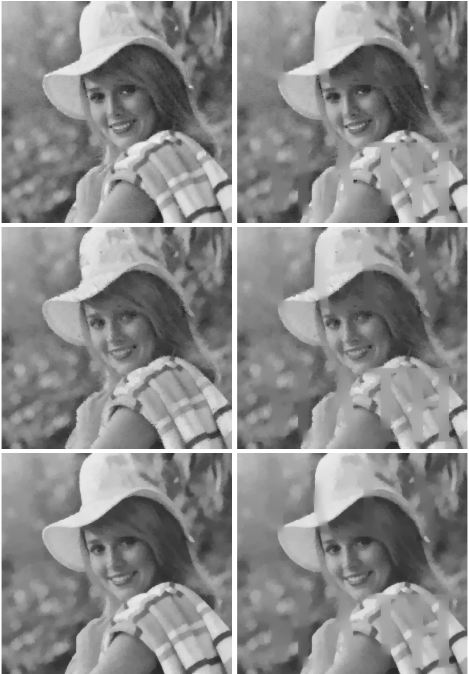
Fig. 7. (Example 2) The minimizer for the energy (8) without (first column) and with (second column) an extra mask. The top, middle and bottom rows show the denoising results with salt-and-pepper, random-valued impulse and addition Gaussian noise.
