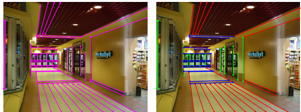
Figure 1. Given a set of lines extracted in calibrated images (left), our goal is to cluster these lines with respect to their (unknown-but-sought) orthogonal vanishing points (right). Each color corresponds to a set of parallel lines.
