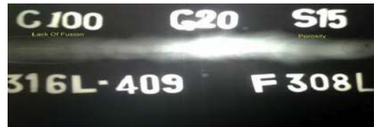
Fig. 4. Radiographic film for sample No.3.
