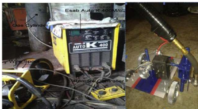
Fig. 1. The photographic view welding set-up.
