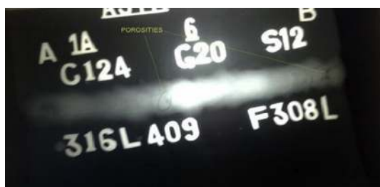
Fig. 9. Radiographic film for sample No.9.
