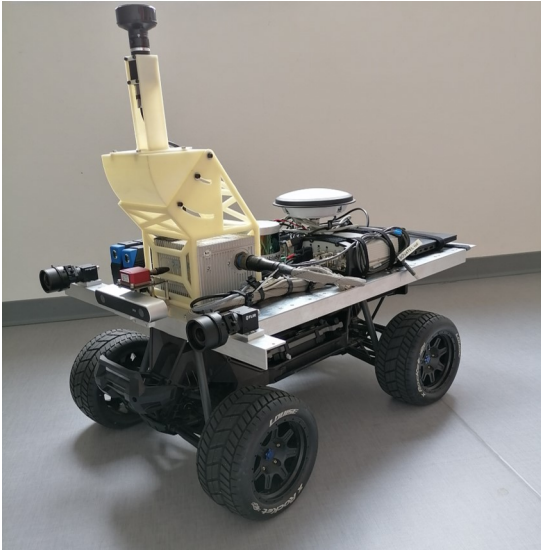
Fig. 1: Our rover setup at ISAE-SUPAERO. The robot is equipped with GNSS receiver and cameras for context ground truth labelling and visual confirmation.
