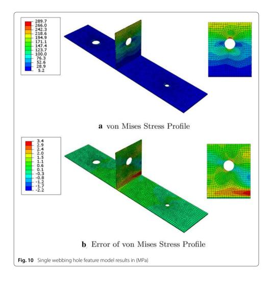
the upper edge, while the single hole has it located on the hole via a stress concentration, occurring at the top of the hole. The second is an almost swirling effect since the side of the hole has low stress that diffuses into the stress field. This is believed to be due partially to the size of the feature. It is believed that if the edge was expanded, there would be a more localized field adjustment as opposed to the mixing/swirling affect seen in Fig. 10a.
