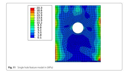
boundary with a maximum of 20.3 MPa compared to 20.7 MPa. However, one difference is that there is a local area of high error near the hole. This localization increases the variation in the confidence interval but is still small compared to the maximum. The fact that the initial design and the single hole design have similar variances is believed to be a trade-off between the Saint-Venant's principle of being far away from the loading and the nature of the stress concentration.
