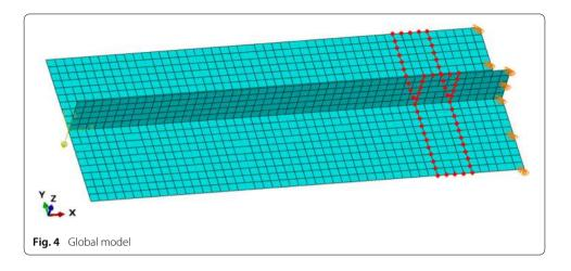
This selection of the applied force is based on the global von Mises stress. The result from the global system reaches a peak stress near the von Mises yield criterion of 265 MPa.
