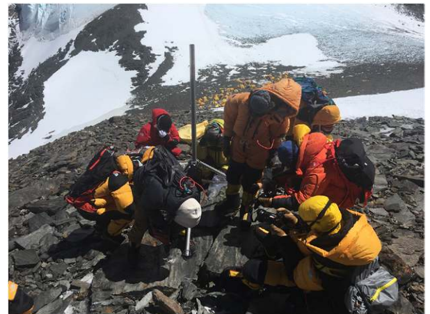
Fig. B2. The South Col AWS being installed. Note the tents of Camp IV in the background, and the exposed glacier ice visible behind. Photo credit: Baker Perry/National Geographic.
