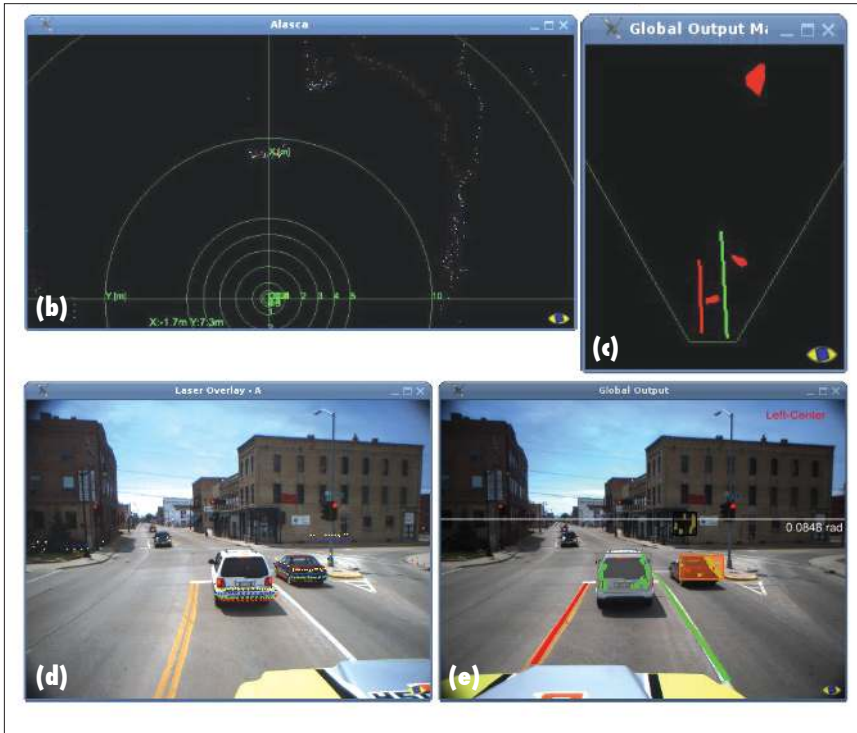
Figure 2. Examples of visual data outputs for the TerraMax prototype vehicle: (a) laser-scanner data, (b) top view of the area in front of the vehicle, showing lane markings and obstacles, (c) laser data mapped on the left camera image, and (d) the final results showing lane markings and obstacles after data processing and sensor fusion in real time.
