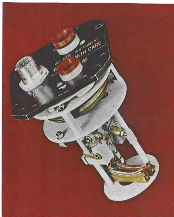
This precision transducer, by Penny and Giles of Christchurch, transmits a continuous reading of air speed to the crash recorder used by most international air lines, the potentiometer converting the movements of a pressure-sensitive diaphragm to electrical signals. It is wound with the high resistivity molybdenum-palladium-gold alloy with a copper-silver-gold alloy wiper
