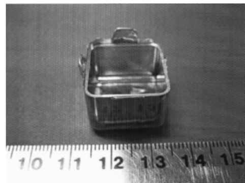
FIG. 3. \text{Au}_{49}\text{Ag}_{5.5}\text{Pd}_{2.3}\text{Cu}_{26.9}\text{Si}_{16.3} , superplastically formed from a rod shape into this article. The forming was carried out in air at 423 K for 200 s under a forming pressure of 100 MPa. The amorphous structure of the plastically formed article was confirmed by DSC and x ray. Note that the as-formed article is shown with no subsequent finishing. The flash and overflows have not been removed.
