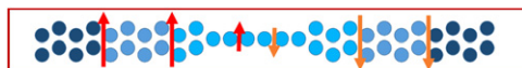
Figure 17. Sketch of the EM setups used in the calculation of spin-resolved transport through nickel electrodes that corresponds to the EM unit cell shown in figure 5. The scattering region is shown in light blue, the first PL is shown in grayish blue, and the second PL is shown in dark blue. The second PL is followed by vacuum.
