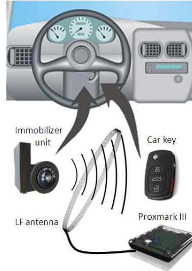
Figure 5: Experimental setup for eavesdropping
