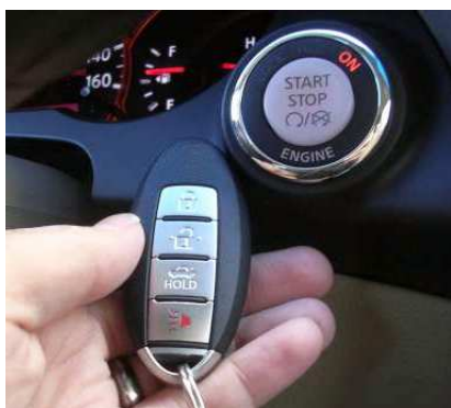
Figure 3: Keyless hybrid transponder and engine start/stop button
