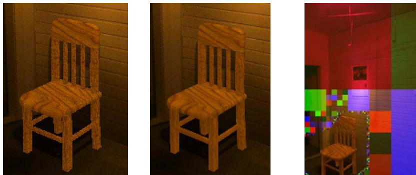
Fig. 6. The left image was generated with standard differential rendering. The middle image was calculated on a higher resolution, the virtual object looks better integrated in the photograph. Right image: Changes in direct light are rapidly identified with the pixel shaft hierarchy. Each colored block represents a region in the photograph without changes in direct light, identified with only one shaft test
