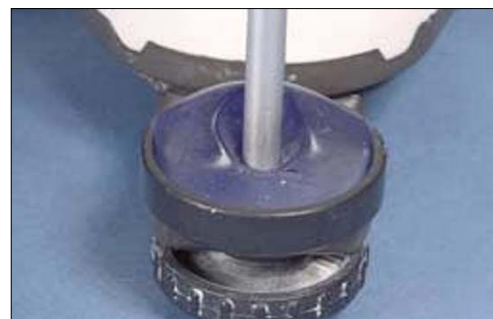
Fig. 13b Custom incisal guidance table. The incisal pin of the articulator is resting in a position that is related to the centric occlusion of the models
