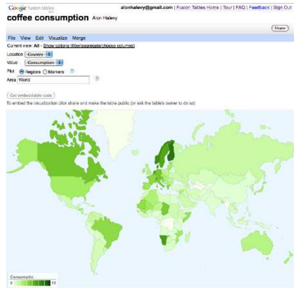
Figure 3: Displaying an intensity map after importing data about coffee consumption. Fusion Tables detects a geo-location column in the data and offers map visualizations.
