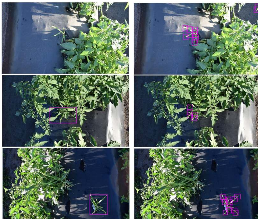
Figure 2. Examples of YOLOv3-tiny network detection of goosegrass ( Eleusine indica ) growing in competition with tomatoes ( Solanum lycopersicum ) using either entire plant (left) or leaf blade (right) annotation techniques in Balm, FL, USA in 2019.
