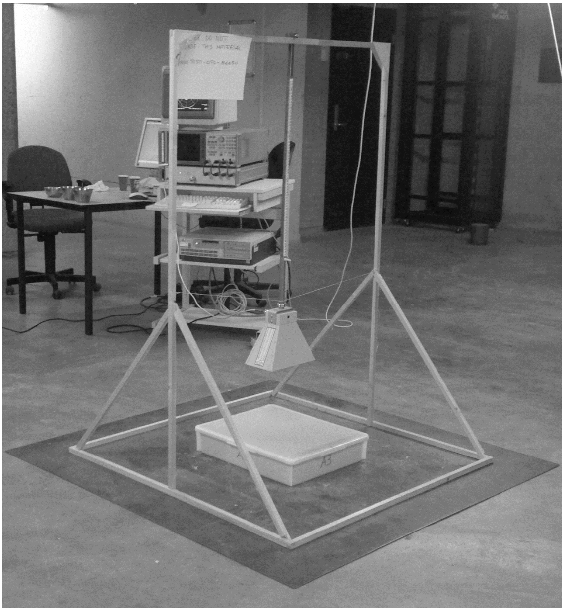
FIGURE 3. Test devices and equipment a) SFCW radar set-up using a vector network analyzer HP 8573C (Hewlett Packard Company, USA) and a linear polarized double-ridged broadband TEM horn BBHA 9120 A (Schwarzbeck Mess-Elektronik, Germany), in a mono-static configuration.
