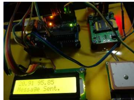
Fig 13: Result for Showing Location of Vehicle on LCD
