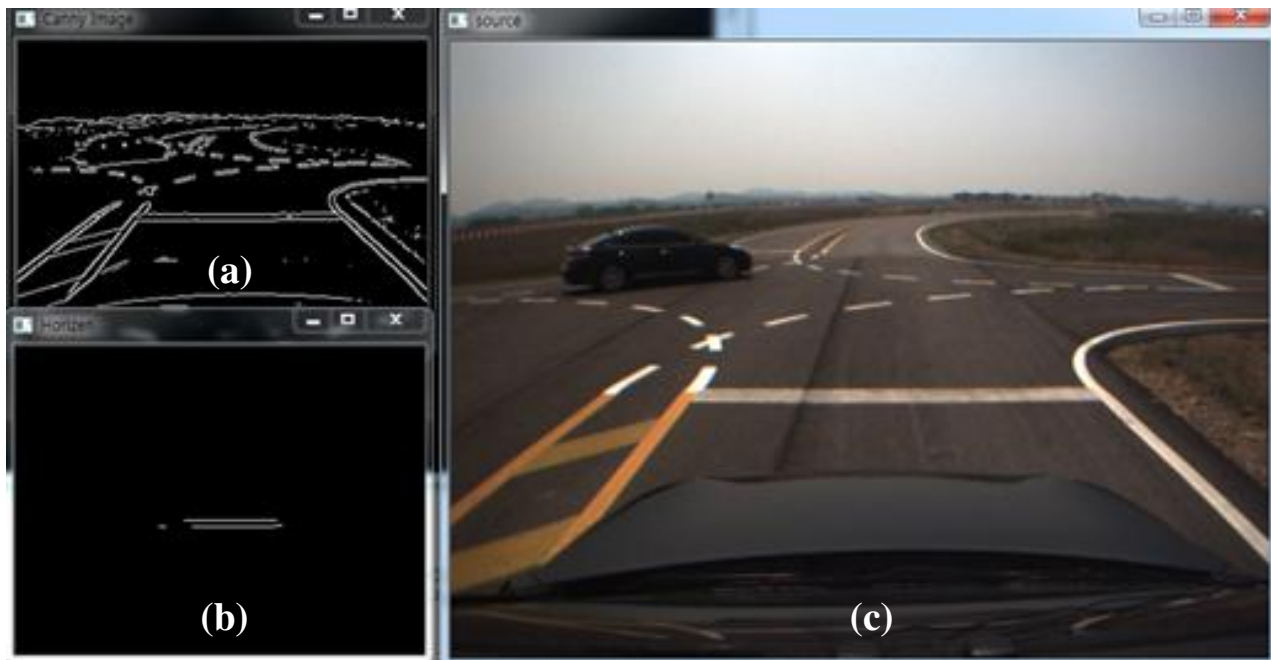
Figure 11. Result of the stop line detection: (a) Canny edge detection; (b) detected stop line; (c) raw image.
