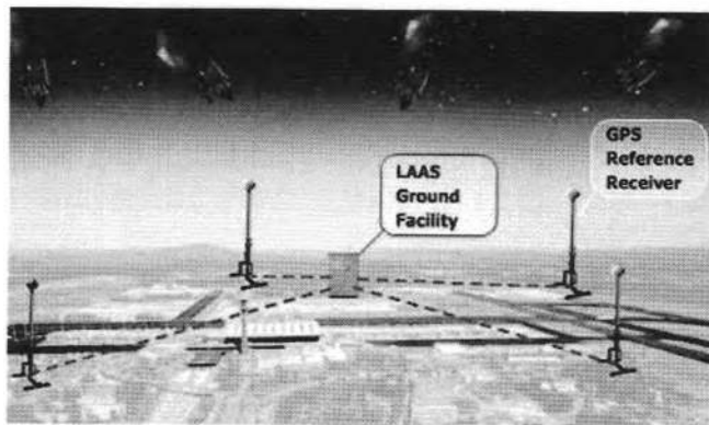
LAAS Ground Facility (LGF) Calculates Errors in GPS Position and Formulates the LAAS Correction Message
