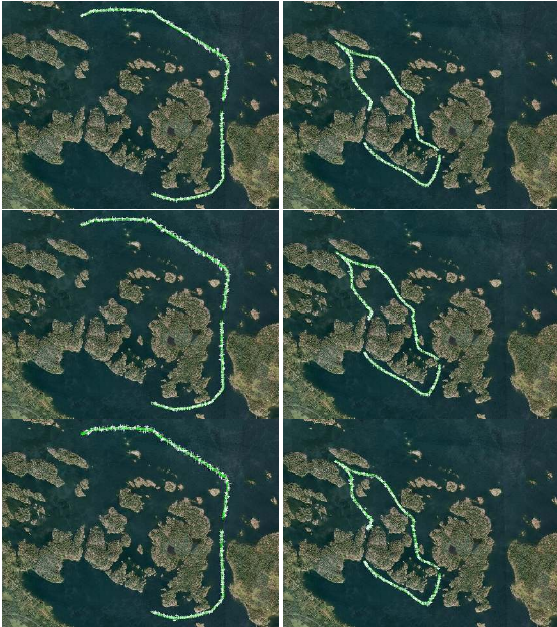
Figure 18: Position estimation results with proposed method (white) and GPS (green). Synthetic FOV 270° (top), 180° (middle), and 120° (bottom). Test day 2 (left) and test day 3 (right). The position estimation accuracy degrades with a narrower FOV as expected.
