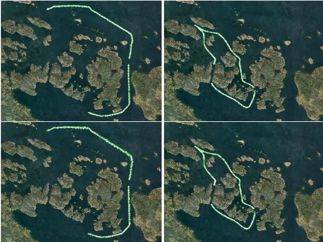
Figure 17: Position estimation results: GPS (green), proposed method (white). MOSSE filter registration (top) and spatial registration (bottom). Test day 2 (left) and test day 3 (right).
