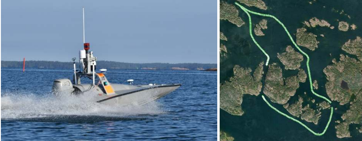
Figure 1: Left: The USV equipped with a Ladybug omnidirectional camera. Right: Test image position estimates with the GPS (green) and the proposed method (white).
